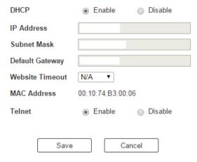
**Enable** DHCP to allow the DHCP server to assign an IP address to the VM6404H. Select **Disable** to enter your own static IP address settings for the device
