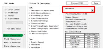
In the **Resolution** drop down menu, choose a resolution with values that fit the attached monitor/display device and click **Save**.
