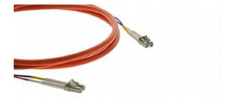
Kramer's 2LC fiber optic cables are constructed of 2 individual color coded multimode 50/125um simplex cables of diameter 2.0mm each, contained in a round orange jacket. They are companions to various Kramer detachable transmitter/receiver sets.
